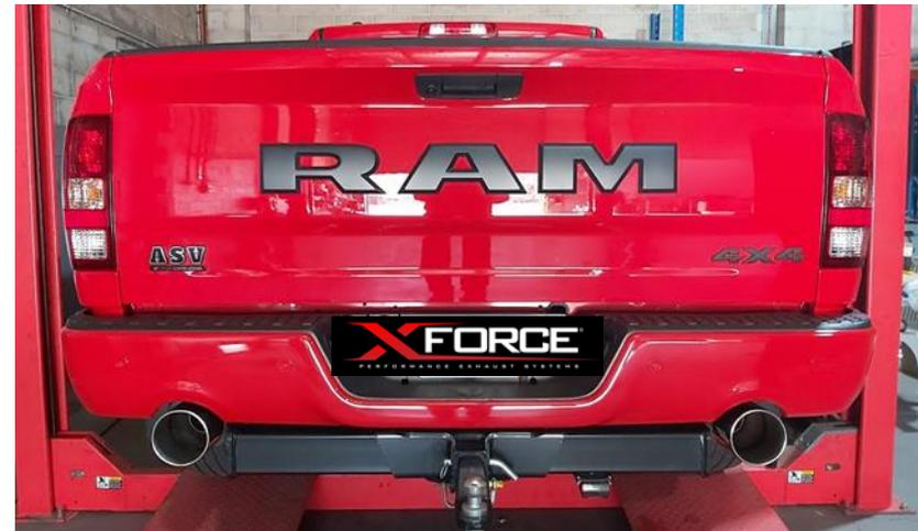
Note: When you first start your vehicle after the installation of your new XFORCE Performance Exhaust System, there may be some smoke and fumes coming from the system. This is a protective oil based coating used in the manufacturing of mandrel bent performance exhaust tubing. This is not a problem and will disappear within a very short period of time after the exhaust has reached normal operating temperatures.
